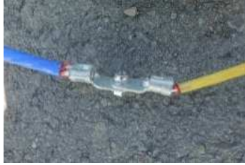
Fig. 6. Terminal extension method.
